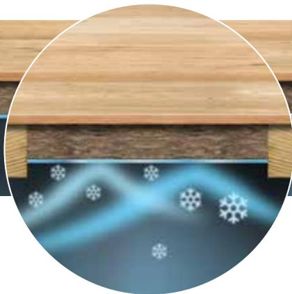
The wind-wash barrier guards against air movement keeping a more consistent temperature inside your home.
